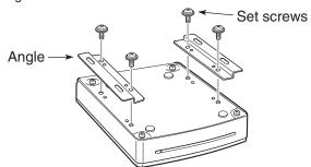
② Mount the receiver securely with the four supplied screws (M5×20 mm) to a flat surface which is more than 10 mm (13/32 inch) thick and can support more than 2 kg (4.4 lb).
